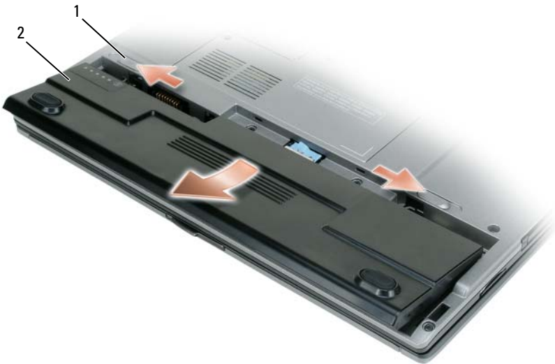
1 battery-bay release latch (2) battery
